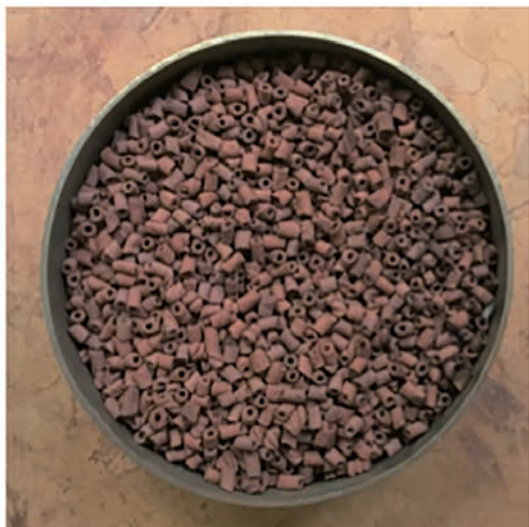
写真5 充填形試作触媒 (FL-1.9-6.0-HM)
