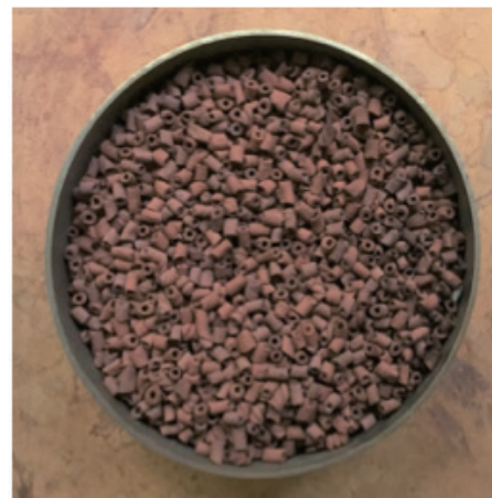
写真5 充填形試作触媒 (FL-1.9-6.0-HM)
